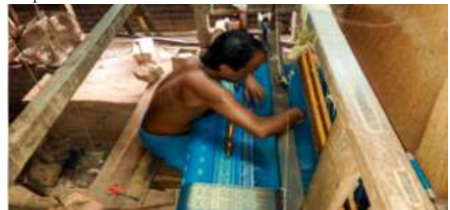
Figure 3.1.1: The saree is being woven in a pit loom with jacquard attachment
